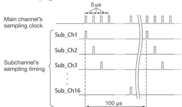
When the number of subchannels to be measured is 2 (subchannels 1 and 16 set to ON)
