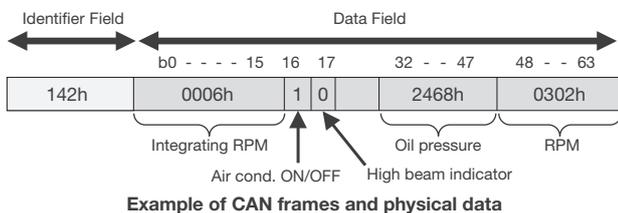
The following is an example of how CAN data can be monitored. With CAN data frames, multiple data (physical data) are carried and received under a single ID. These modules acquire (extract) identifiers for data fields defined as channel settings (for example, "oil pressure" or "RPM"), re-sample the data, and then convert it to time series data.
