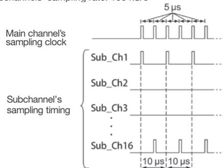
For example, if the main channel's sampling rate is 200 kS/s, the sampling clock is 5 μs period. The subchannels are sampled at this sampling clock in turn. Therefore, the subchannel's sampling timing is as shown in the figure above. Because scanning all required channel's takes time in proportion to the number of subchannels to be used (set to ON), the greater the number of subchannels to be used, the lower the sampling rate for one subchannel.
