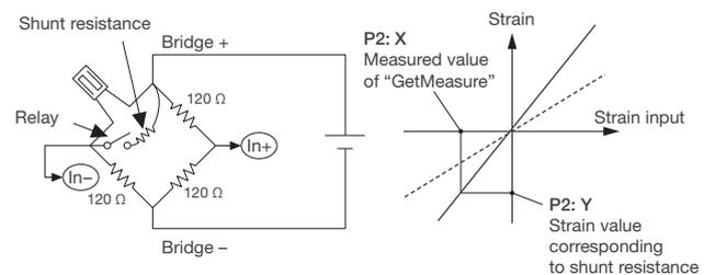
The model 701271 Strain Module (DSUB, shunt CAL) supports shunt calibration. A bridge head that supports shunt CAL (model 701957 or 701958) is required to execute shunt CAL.
