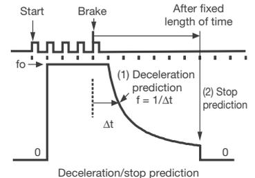
You can detect actions from pulse output stop (break, etc.) to the actual stop, therefore it is effective for applications involving pulse measurement associated with deceleration and stopping.
