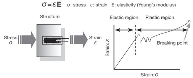
Stress is calculated using the relationship of elasticity (Young's modulus), which depends on structure's material, and the durability of the structure.
