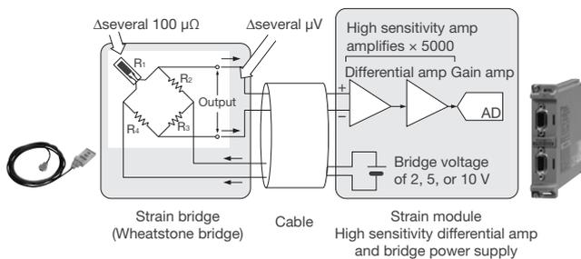
Furthermore, because the bridge output is as small as a few micro volts, the input must be amplified inside the strain module using a differential and high gain amp.
